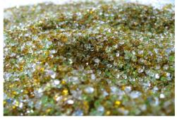
It is particularly favoured for use in environmentally sensitive locations. The glass manufacturing process fixes the free crystalline silica responsible for silicosis. As a result, any dust generated when using graded glass abrasive is virtually free of crystalline silica and is classified merely as a 'nuisance dust'.
